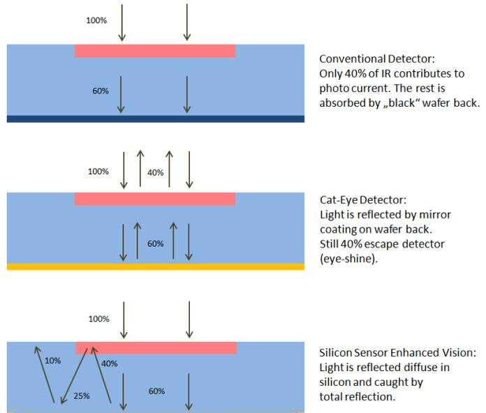
Fig.2: Mechanisms of IR absorption in Silicon
